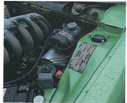
● Check where the front panel joins inner wing
