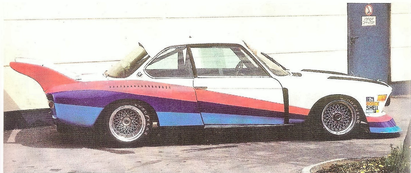
The Group 5 turbo-charged CSL at the factory, a new 'cow-catcher' front spoiler was matched to a sweeping extended rear wing
